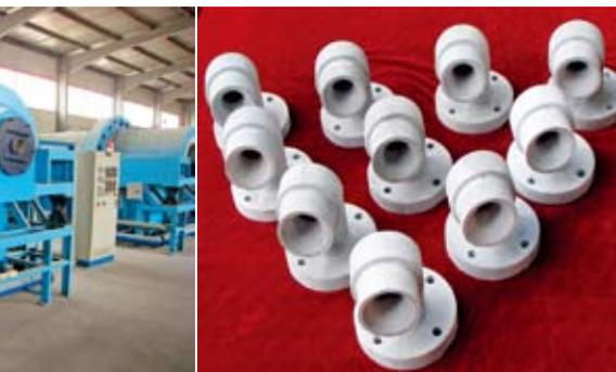
脱硫装置用的Si<sub>3</sub>N<sub>4</sub>-SiC雾化喷嘴
